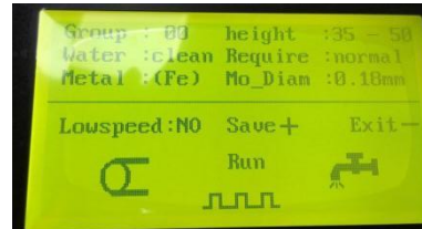
Pic. 13 Operation panel_ Mo Drum & Water pump prepared
