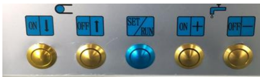
Pic. 11 Button of Mo Drum & water pump
